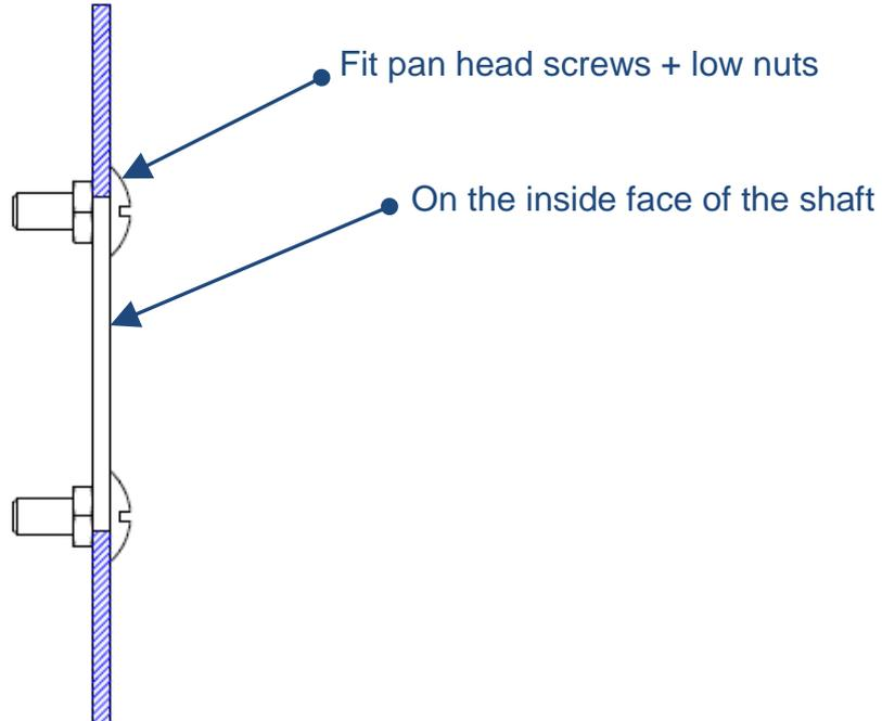
3) Adjust the triggering distance of the VIGIBELT® TOUCH sensors. This distance is the dimension between the inside face of the elevator and the contact face of the sensor.
